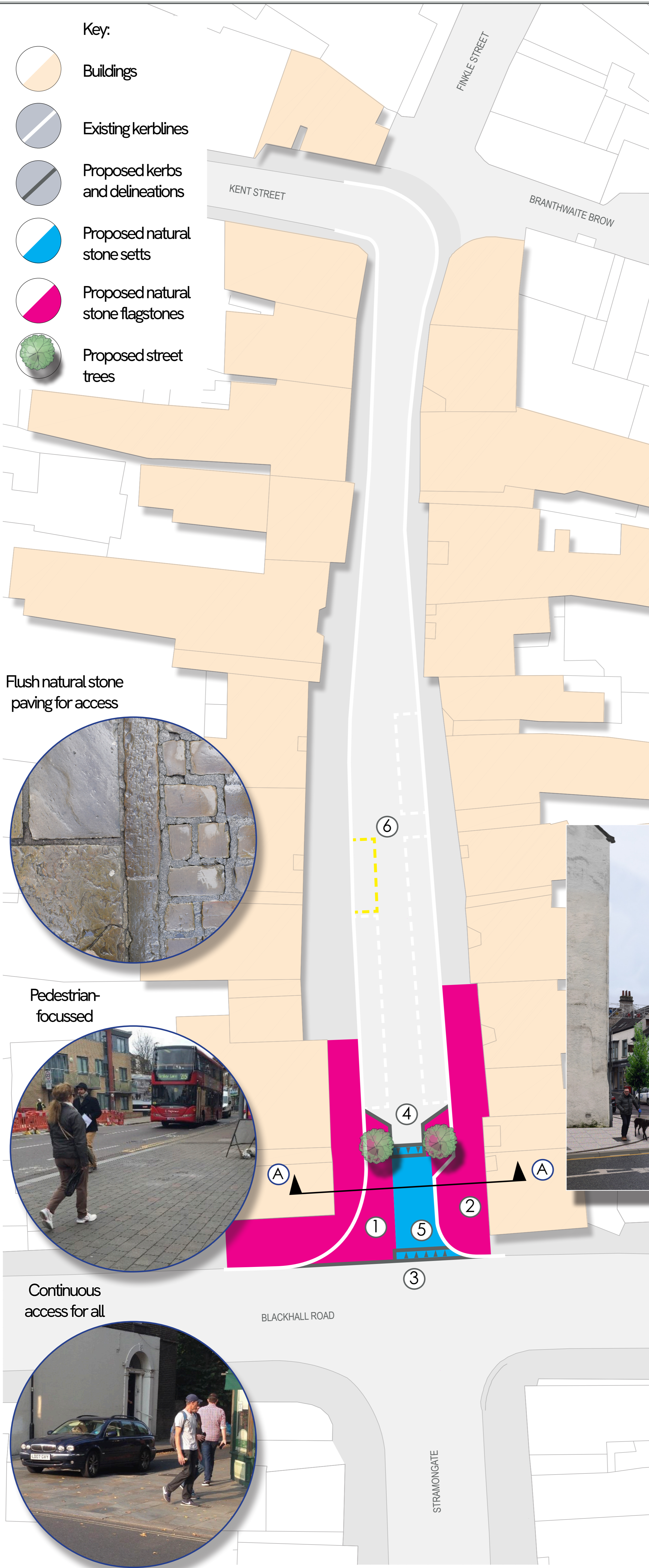
A Continuous footpath section illustrating the proposed surface arrangement, street trees and existing on-street parking beyond.
