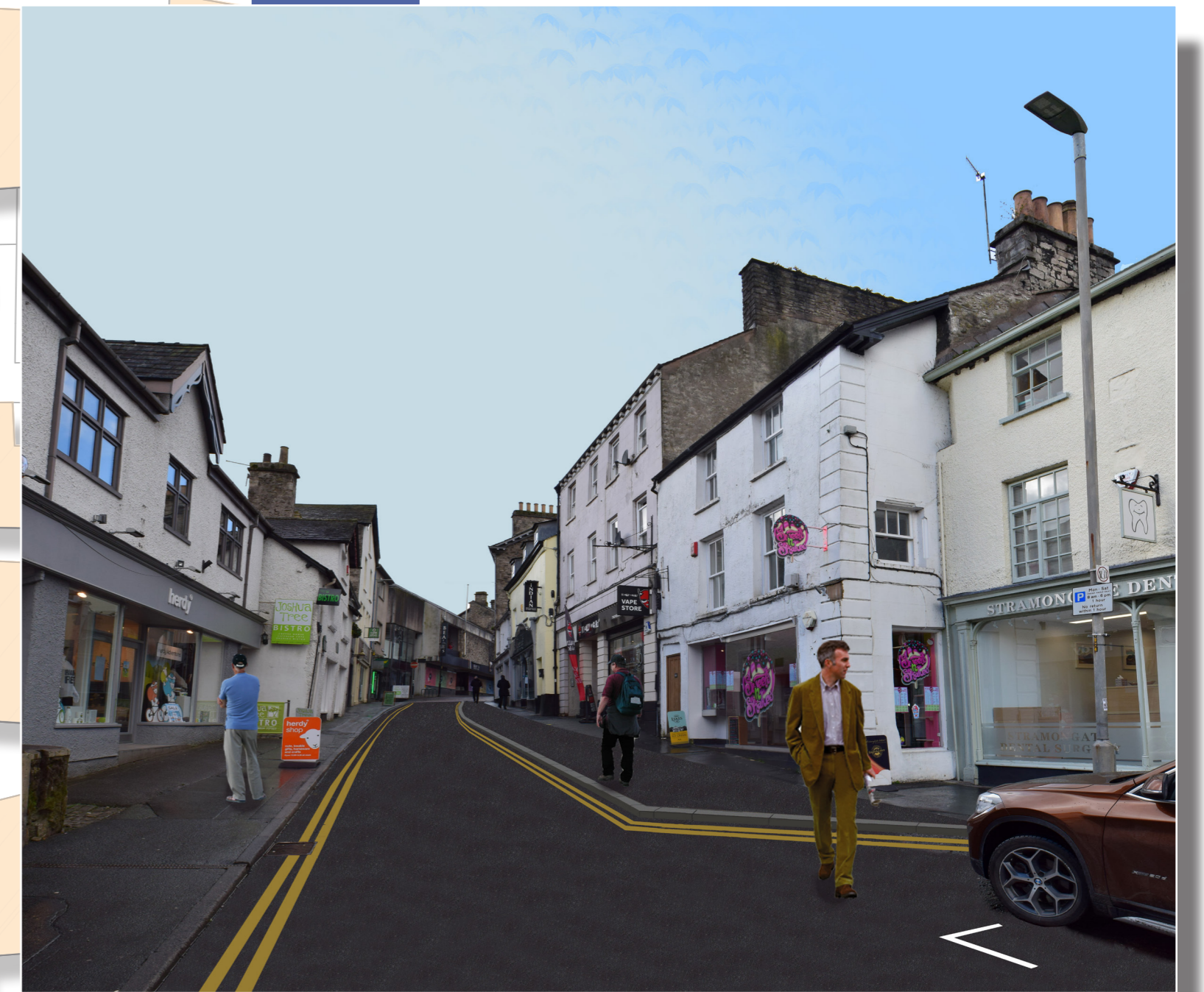
Above: Artist's impression of Option 1 illustrating the proposed widened footpath and narrow carriageway at existing levels
